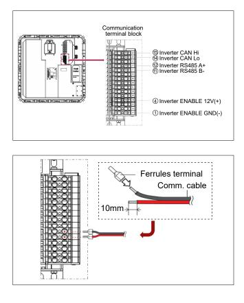
1. Find the Communication terminal block inside the terminal hole.
