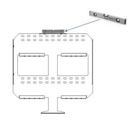
Fasten the Mounting Brackets with M6 bolts.
