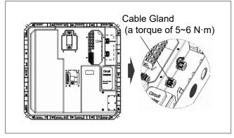
1-2. Or seal the Cable gland with sealant after fasten the Cable Gland.
