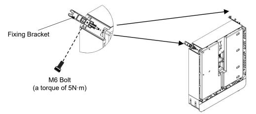
2) Move the first BMA to the wall and mark the drill point for the Fixing Brackets. Drill holes at the marked points and fix the BMA to the wall.
