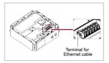
Insert the Ethernet cable through the gland hole and connect the cable it to the Terminal for Ethernet cable.
