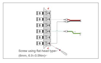
1. Find the Power terminal block inside the terminal hole
