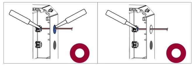
※ IP55 is not met when only outer hole is sealed. Make sure that inter hole of the Cable Gland is sealed properly.
