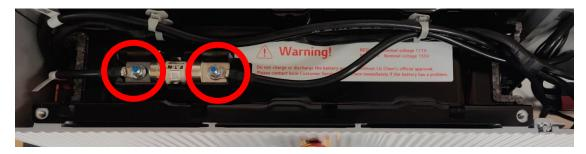
Measure at these points with the **negative terminal** of your measuring device. Please measure before and after the fuses to check if the fuse is not defective.
